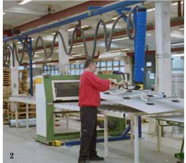
2. Large and very thin steel plates are moved through this filmcoating machine.
