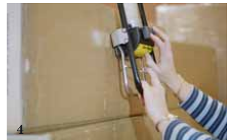
4. The optional remote control has quickly become a frequent request allowing the operator to control the vacuum pump without having to leave the operating area. Available with all units.
