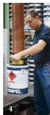
4. A VacuEasylift that lifts drums/tins/buckets is a popular installation in the pharmaceutical/chemical industries. We deliver suction feet for handling one or more tins at a time.
