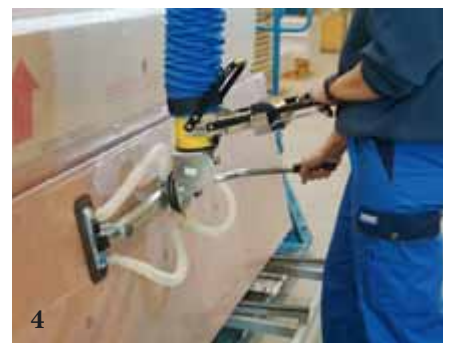
3-4. This system covers an area of in all 5 working stations. An angle adapter with handle is used to turn the suction foot 90 degrees and lift the panels from vertical to horizontal position.
