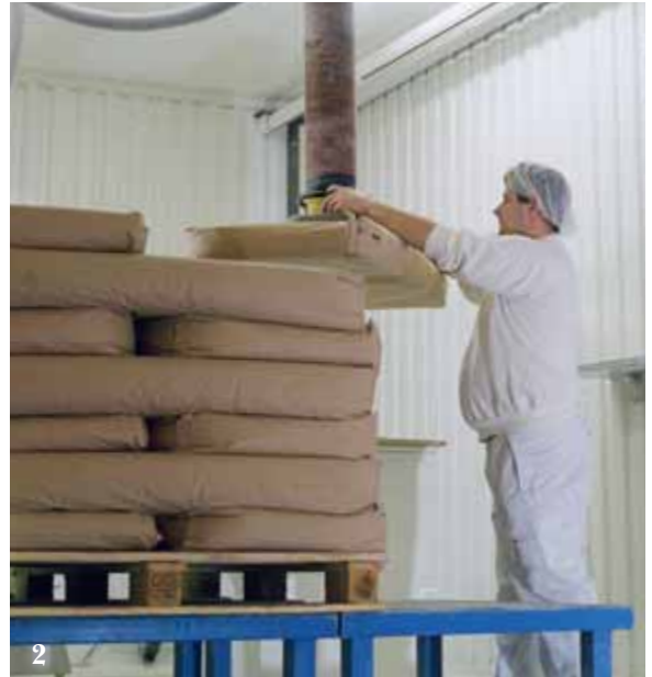
1-2. Manual bag handling is extremely heavy and has therefore become one of the top ten most popular applications with VacuEasylift. The VM160 handles bags up to 60 kg which covers practically all bags handled in food and chemical industries.
