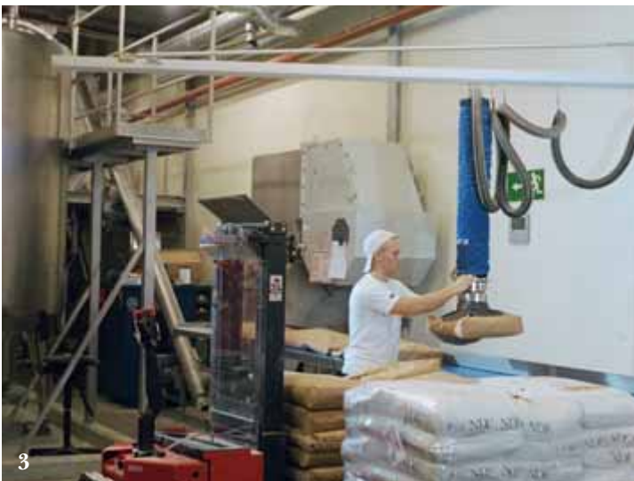
1-2. Manual bag handling is extremely heavy and has therefore become one of the top ten most popular applications with VacuEasylift. The VM160 handles bags up to 60 kg which covers practically all bags handled in food and chemical industries.
