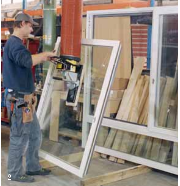
1-2. The suction feet to lift panels and boards vary in design due to variations in size, weight and density of material. In some cases two suction feet on a wide yoke is sufficient. This also applies to all types of window handling.
